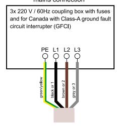
The tanning device is by default set up to operate on 3 phases but it can be changed over to 2-phase operation. The wiring for 3-phase operation is shown below:
