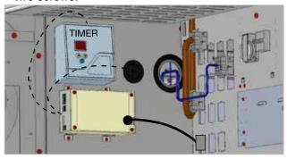
Connect the external cable and the timer to the T-Max box.
