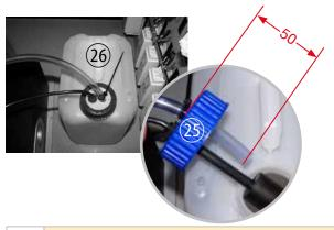
Unscrew the closing lid of the condensate canister.
