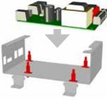
Attach the connectors to the T-Max board and housing (ground).
